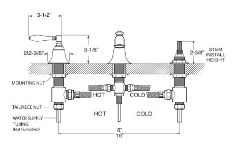
NOTE: Spout and valves install through 1-1/4" diameter holes
