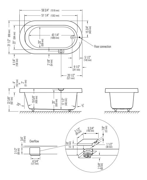
$<sup>^{*}\</sup>mathrm{A}$  bathtub fitted with back jets can cause the pump to protrude by approximately 3" from the overall dimension.
