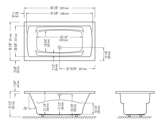
$<sup>^{\</sup>star}\mathrm{A}$  bathtub fitted with back jets can cause the pump to protrude by approximately 3" from the overall dimension.
