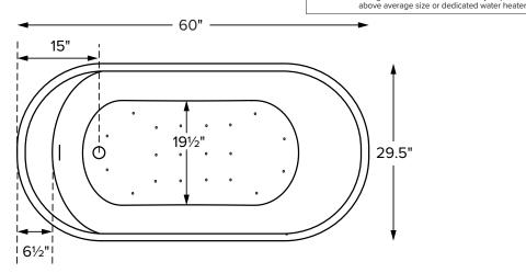
The Eryn features a flat deck on the drain side for mounting faucetry.
