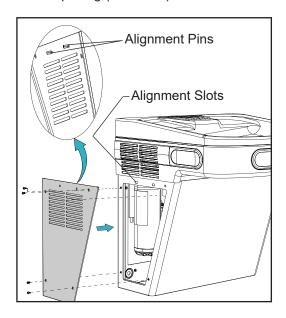
Once the access panel is set in place, refasten the (4) security Torx screws bits starting by hand and firmly secure each screw in place.
